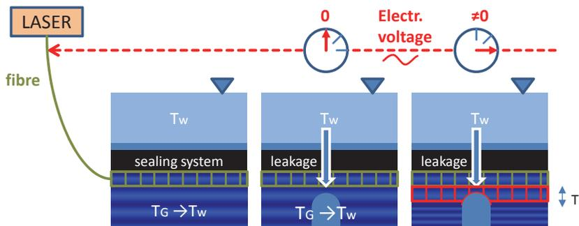
Figure 2.7. Heat-pulse method for leakage detection [101].
