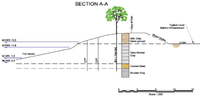
Figure 2.10. Boston dike cross section A-A [114].
