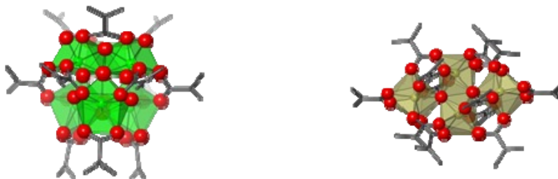
Figure 4. Schematic of Zr-based (left) and Hf-based (right) oxoclusters structures. Green (left) or brown (right) polyhedron delimits the coordination geometry of Zr and Hf atoms, respectively. Red balls represent oxygen atoms and gray bars represent carbon-carbon bonds.
