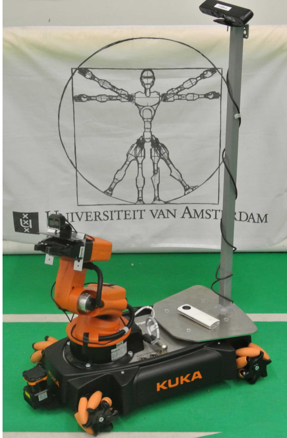
Figure 1. The Kuka youBot mounted with all its sensors: Asus Xtion Pro Live, Hokuyo UTM-30LX and a Microsoft LifeCam HD-5000.
