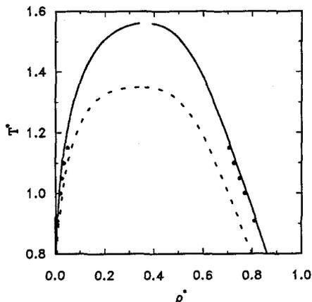
Figure 1. Comparison of the Gibbs-ensemble simulations of the Lennard-Jones fluid with density-dependent potentials ( $a=0.1$  and  $b=1$ , dots) with the prediction of the equation of state (solid line). For comparison, the phase diagram of the Lennard-Jones fluid  $a=0$  and  $b=1$  is also shown (dashed line).
