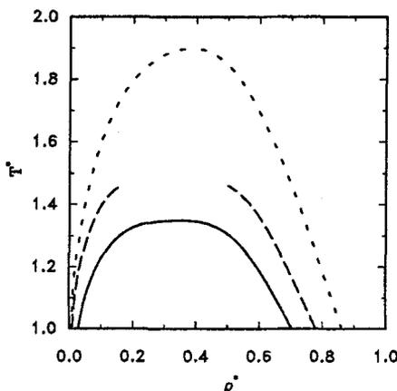
Figure 2. Phase diagram of the Lennard-Jones fluid with density-dependent potential,  $a = 0.25$  and  $b = 1.0$  (dotted line). The dashed line is the phase diagram that would have been obtained with Gibbs ensemble simulations using the assumptions of ref. [9]. The solid line gives the phase diagram of the ordinary Lennard-Jones fluid.
