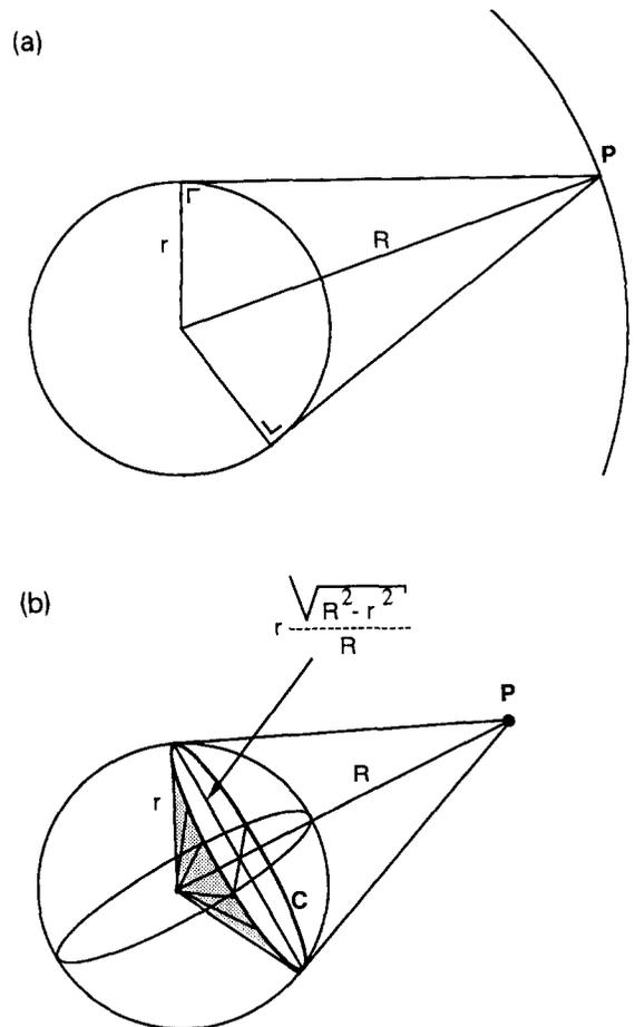
Figure 4. (a) In two dimensions the point  $P$  contributes at two points to the distribution  $p(r)$ . (b) In three dimensions the contribution of point  $P$  to the distribution  $p(r)$  is proportional to the circumference of circle  $C$ .
