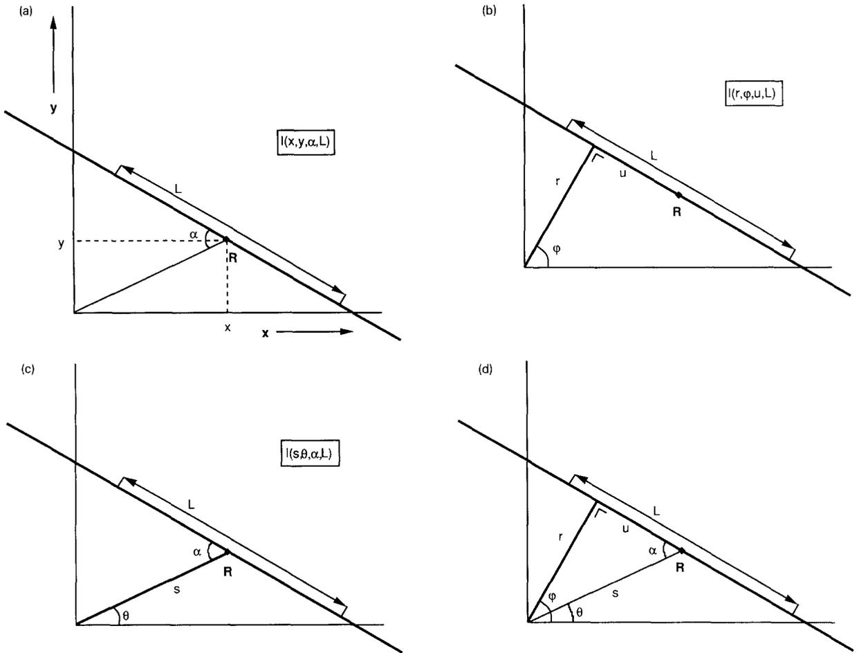
Figure 1. (a) A straight line segment in cartesian representation. (b) A straight line segment in normal representation. (c) A straight line segment in polar representation. (d) The relation between the polar and normal representations.
