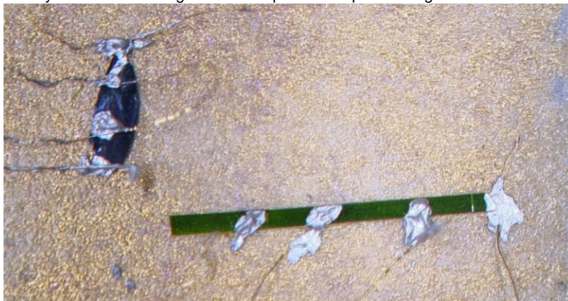
Figure S34. Photo of the crystals mounted on a PPMS resistance puck in a four-point geometry seen through a microscope. Top left: \{(p\text{MeOPh})_3\text{N}\}_2\{\text{DDQ}\}_3\{\text{CD}_3\text{CN}\}_4 . Bottom right: \{(p\text{BrPh})_3\text{N}\}\{\text{DDQ}\}_2 . For scale: the green crystal is 6 mm long.
