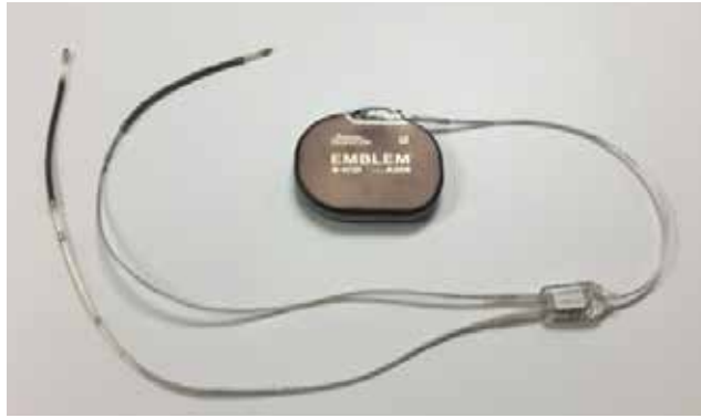
Figure 2 Photo illustrating how the dual electrode configurations tested in the study were realized using an EMBLEM S-ICD, an investigational Y-adaptor, and two S-ICD electrodes.
