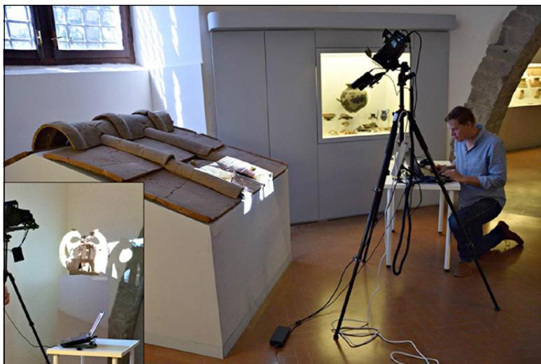
Fig. 5 – Scanning the roof and acroterion of House B in the Viterbo Museum.
