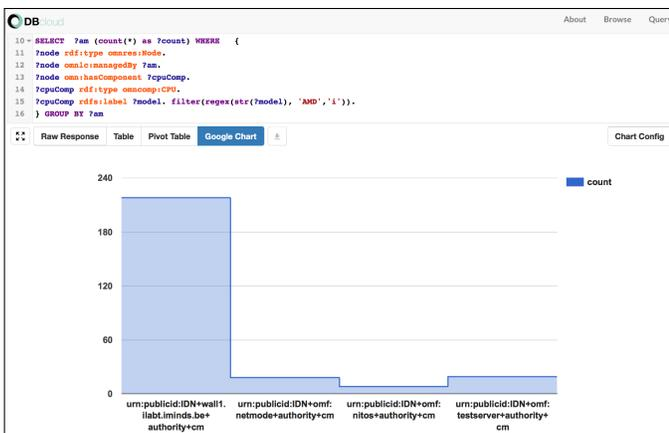
Fig. 4: Finding testbeds containing nodes with AMD hardware
