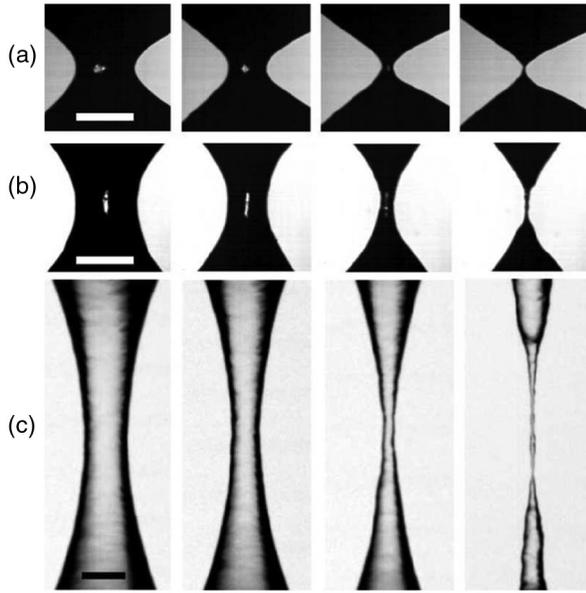
FIG. 1. Liquid bridges and detaching drops of a 2% Carbopol solution at different extension velocities  $V$  and times to breakup  $\tau$ : (a)  $V = 0.018$  mm/s at  $\tau = 3.59, 1.2, 0.08,$  and  $0.0001$  s. (b)  $V = 1.8$  mm/s at  $\tau = 0.15, 0.065, 0.0095,$  and  $0.0001$  s. (c) Droplet breakup at  $\tau = 0.0067, 0.0035, 0.0005,$  and  $0.0001$  s. The scale bar is  $500 \mu\text{m}$ .
