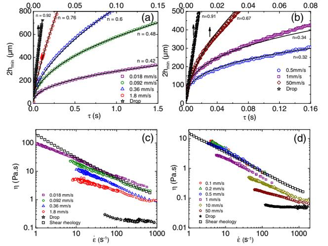
FIG. 2 (color online). [(a),(b)] Minimum neck diameter  $2h_{\min}(\tau)$  for different values of  $V$ . Fits are power laws with exponent  $n$ : The faster stretching rates have their time scale indicated on the upper axis (vertical arrow). [(c),(d)]  $\eta_s$  versus  $\dot{\epsilon}_M$  for different  $V$  values along with the rheology. Fluids used: (a), (c), 2% Carbopol dispersion; (b), (d), 74% castor oil emulsion.
