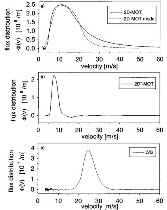
FIG. 2. Velocity distributions  $\Phi(v)$  of the flux. (a) Comparison of 2D-MOT and our simple model, (b) 2D<sup>+</sup>-MOT, (c) LVIS. The data are obtained by taking the derivative of the time-resolved photomultiplier signal [Eq. (1)]. The curves were measured at different background pressure in order to optimize the respective flux [Fig. 3(a)]. The small dip towards negative flux in (b) around  $v = 17$  m/s is an artifact resulting from a fluctuation of the time-of-flight signal.
