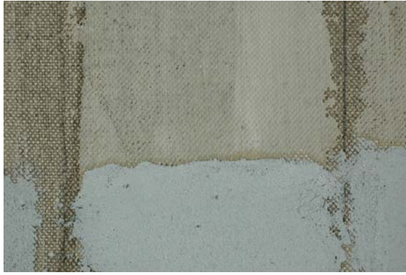
Figure 12.8 Halo formation in section 6.3: wheat seed starch with pipe clay ground layer, covered with grey oil paint (lead white, carbon black, linseed oil)
