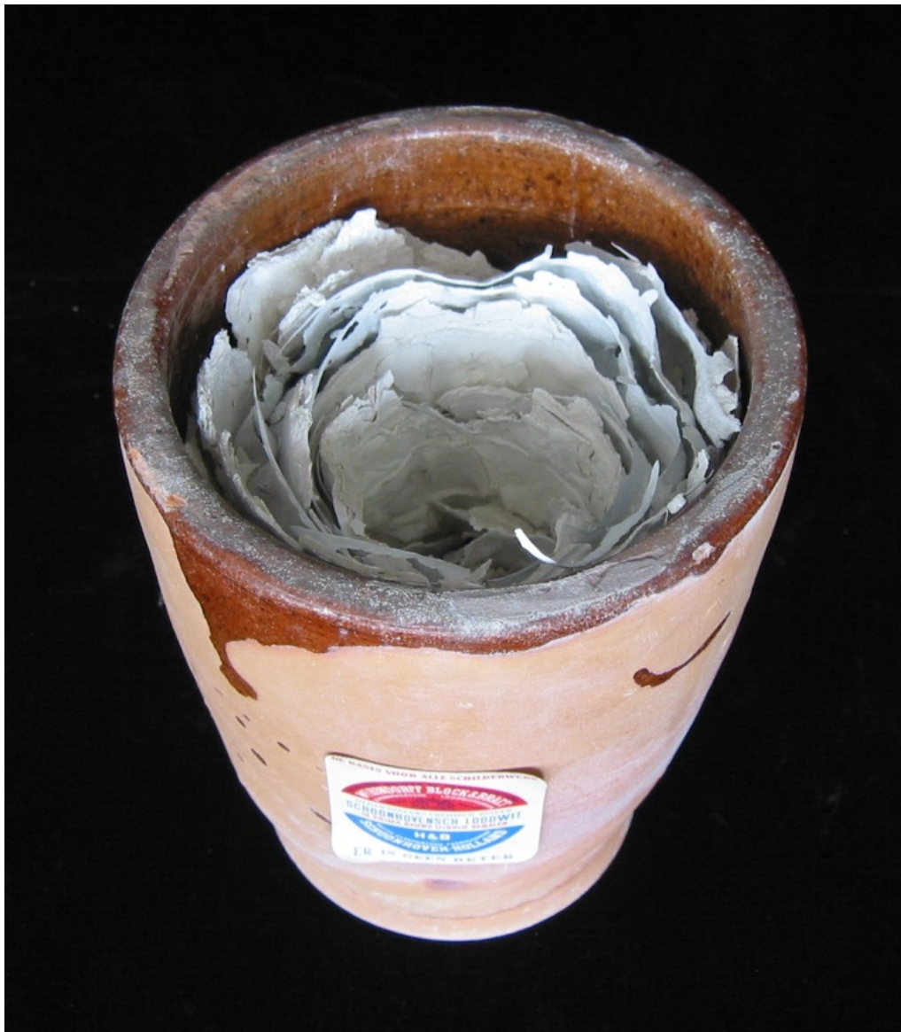
Figure 13.1 Lead white flakes in a stack-process corrosion pot from the Schoonhoven Factory
