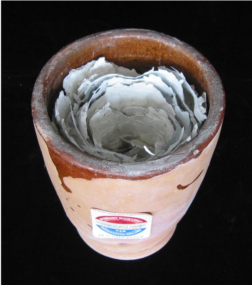
*Figure 13.1 Lead white flakes in a stack-process corrosion pot from the Schoonhoven Factory*
