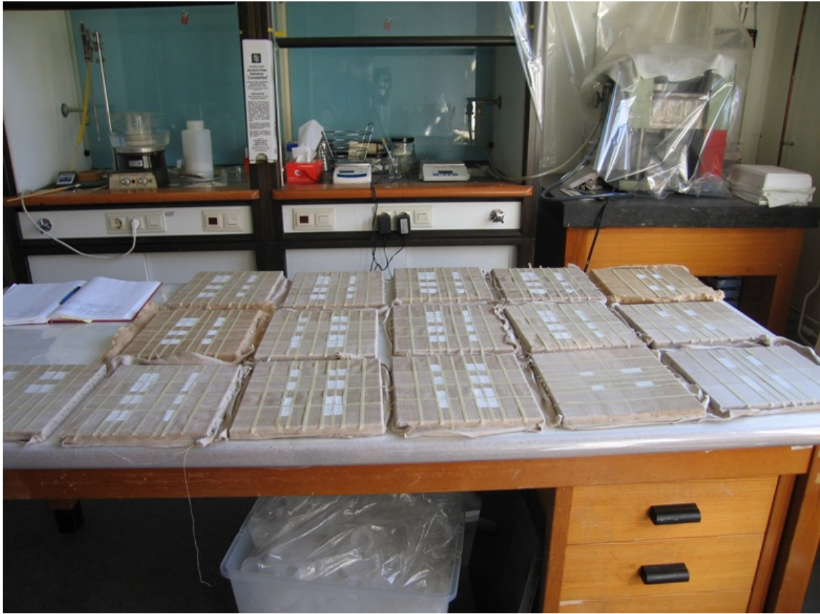
Figure 16.1 Reconstructions of animal glue size layers, the topic of Chapter 11.
