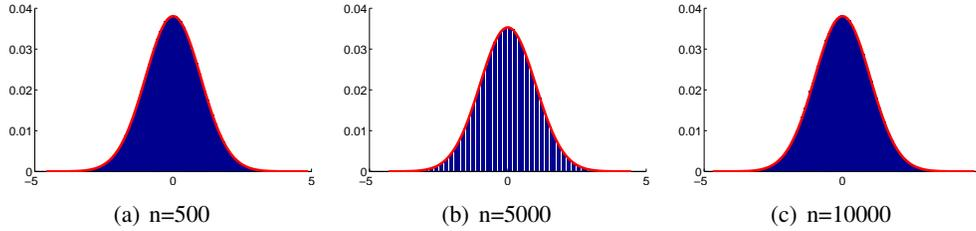
**Figure 1:** Theoretical (red line) and empirical distribution (blue bars) of the t-statistic under resampling  $n$  datapoints without replacement from a dataset composed of digits 7 and 9 from the MNIST dataset (total  $N = 12214$  points).
