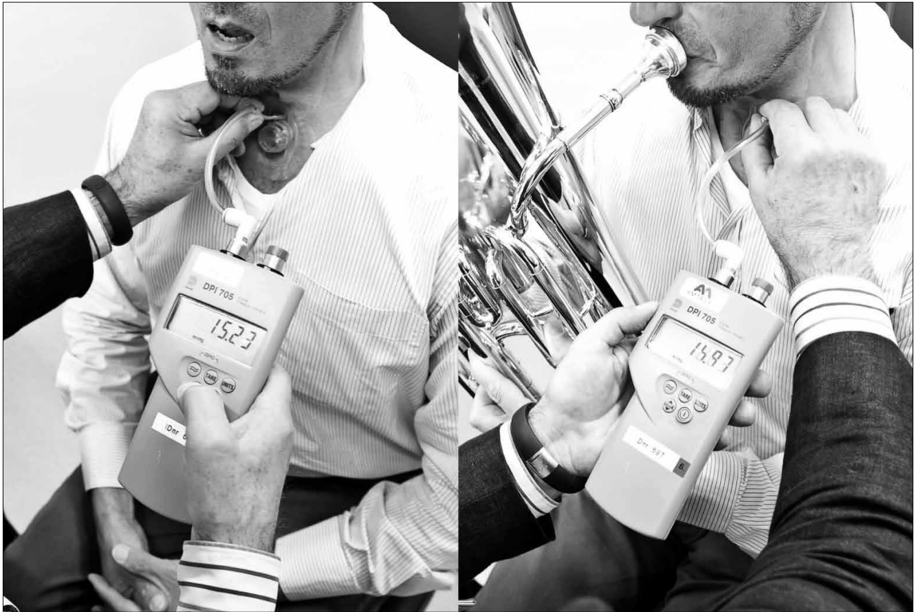
Fig. 1. Trachea pressure measurement during voicing (left), and during brass instrument play (right) using a digital manometer airtight attached into a peristomal adhesive; printed with permission.
