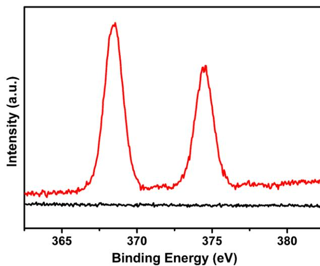
**Fig. S3.** Comparison of Ag(I) XPS of MIL-101-Cr-SO<sub>3</sub>H (black) and MIL-101-Cr-SO<sub>3</sub>Ag (red).
