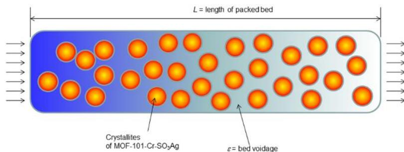
**Fig. S8.** Schematic of a packed bed adsorber. The parameter values used in the simulations presented here are:  $L = 0.12$  m; voidage of bed,  $\varepsilon = 0.75$ ; interstitial gas velocity,  $v = 0.003$  m/s, superficial gas velocity,  $u = 0.00225$  m/s.
