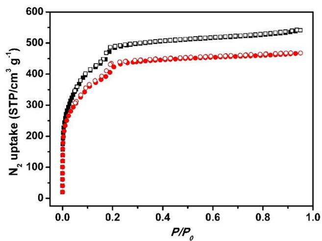
**Fig. S2.** Comparison of N<sub>2</sub> sorption MIL-101-Cr-SO<sub>3</sub>H (black), MIL-101-Cr-SO<sub>3</sub>Ag (red).
