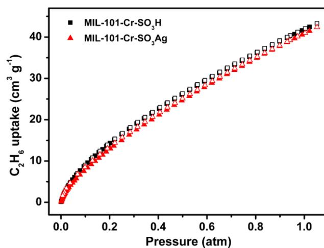
**Fig. S4.** Comparison of ethane sorption isotherms of MIL-101-Cr-SO<sub>3</sub>H (black), and MIL-101-Cr-SO<sub>3</sub>Ag (red) at 296 K.
