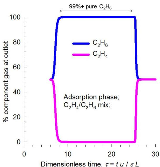
**Fig. S10.** %  $C_2H_6$  in the outlet gas of an adsorber bed packed with MIL-101-Cr- $SO_3Ag$  in the adsorption cycle. The inlet gas is maintained at partial pressures  $p_1 = p_2 = 50$  kPa, at a temperature of 296 K.
