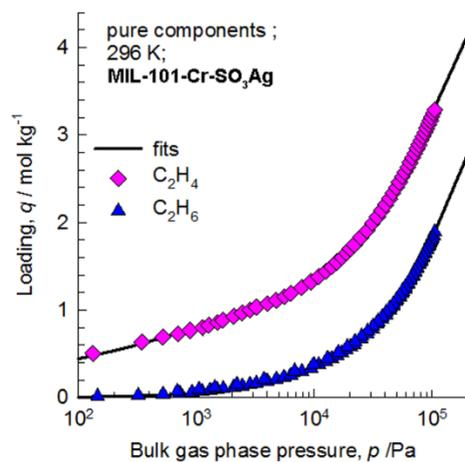
**Fig. S7.** Comparison of the experimentally determined component loadings for  $C_2H_4$ , and  $C_2H_6$  on MIL-101-Cr-SO<sub>3</sub>Ag at 296 K with the isotherm fits using parameters specified in Table S1.
