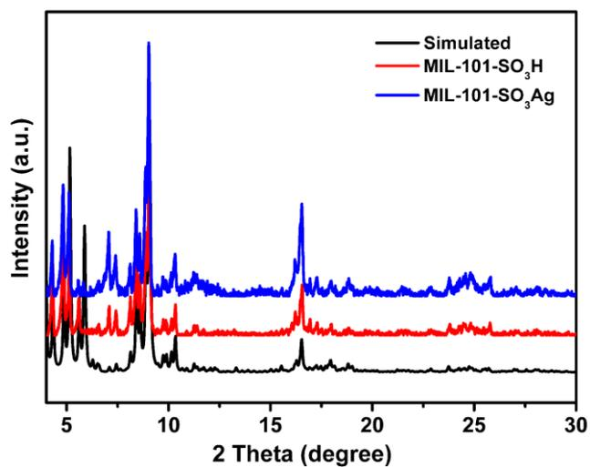
**Fig. S1.** Comparison of XRD of simulated MIL-101-Cr-SO<sub>3</sub>H (black), MIL-101-Cr-SO<sub>3</sub>H (red), and MIL-101-Cr-SO<sub>3</sub>Ag (blue).
