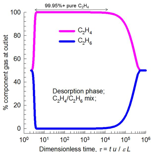
**Fig. S11.** % C<sub>2</sub>H<sub>4</sub> in the outlet gas of an adsorber bed packed with MIL-101-Cr-SO<sub>3</sub>Ag in the desorption cycle. The contents of the bed, that is equilibrated at partial pressures  $p_1 = p_2 = 50$  kPa, at a temperature of 296 K is purged by inert gas. For the calculations presented in the graph, the inert gas is not included in the calculation of the % compositions.
