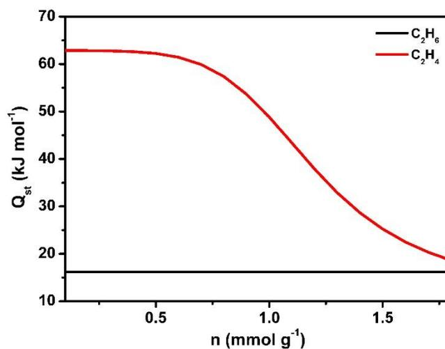
**Fig. S6.** Comparison of isosteric heats of adsorption for ethylene (red) and ethane (black) in MIL-101-Cr-SO<sub>3</sub>Ag.
