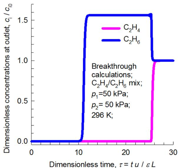
**Fig. S9.** Transient breakthrough of an equimolar  $C_2H_4/C_2H_6$  mixture in an adsorber bed packed with MIL-101-Cr- $SO_3Ag$  in the adsorption phase of a PSA operation. The inlet gas is maintained at partial pressures  $p_1 = p_2 = 50$  kPa, at a temperature of 296 K.
