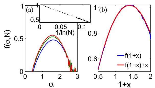
FIG. 5. SFD in 3D at  $E = -1$  for  $\rho = 0.1$ , presenting a parabolic form: (a) SFD for  $N = 10000$  (lower curve),  $N = 30000$  (middle curve), and  $N = 60000$  (upper curve). The inset shows  $f(\alpha, N)$  at  $\alpha = 1.5$  [where  $f(\alpha)$  is maximum] versus  $1/\ln(N)$ . (b) Extrapolation of SFD for  $N \rightarrow \infty$  that fulfills the symmetry  $f(1+x) = f(1-x) + x$  characteristic of NEE states.
