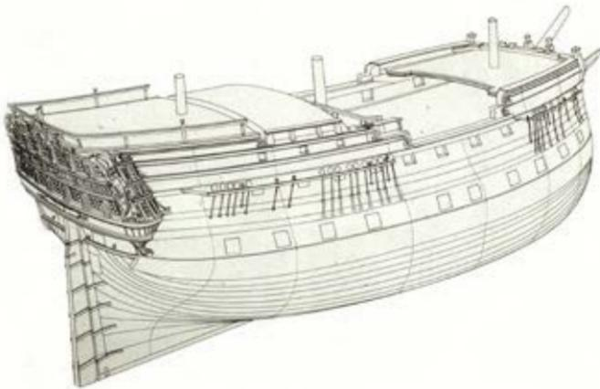
*Fig. 6. Perspective drawing of the hull a VOC-ship of the 150 feet class from the 1740s, based on the contemporary design (drawing R. van Silfhout, Stichting VOC schip Amsterdam).*
