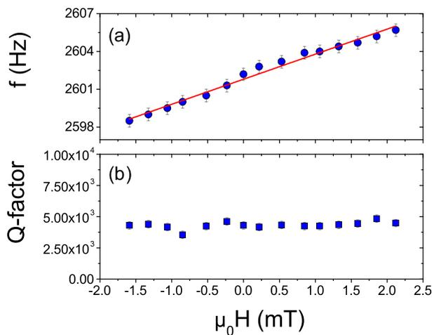
FIG. 4. (a) Resonance frequency as a function of the external magnetic field determined from the cantilever's thermal spectrum. The slope of the curve implies a magnetic moment of  $1.1 \pm 0.1 \times 10^{-12}$  A m<sup>2</sup>, which means a volume of  $0.8 \pm 0.1 \mu\text{m}^3$  has been damaged by the FIB. (b) The quality factor as a function of the external magnetic field as determined by a ring-down measurement.
