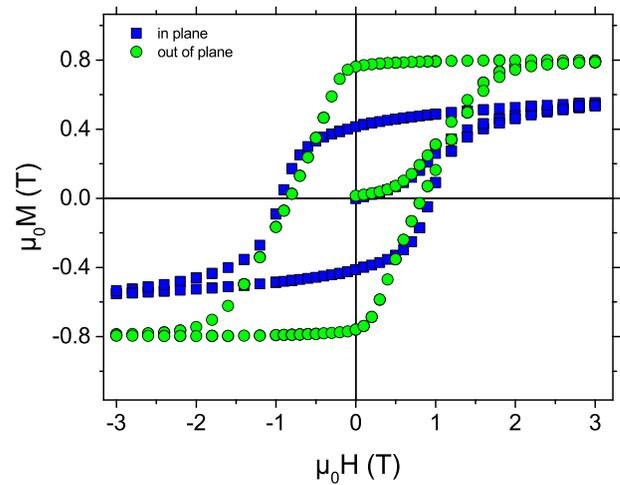
FIG. 3. Magnetization of the film as a function of external magnetic field strength for two different orientations of the sample. For the out-of-plane orientation, the remanent field  $\mu_0 M = 0.76 \pm 0.03 \text{ T}$  and for the in-plane orientation it is  $\mu_0 M = 0.50 \pm 0.03 \text{ T}$ .
