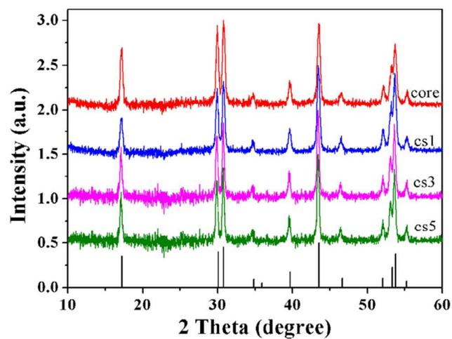
**Figure S1.** X-ray diffraction patterns of NaYF<sub>4</sub>: Yb<sup>3+</sup>, Er<sup>3+</sup> core and NaYF<sub>4</sub>: Yb<sup>3+</sup>, Er<sup>3+</sup>/NaYF<sub>4</sub> core-shell UCNPs. The standard diffraction pattern of hexagonal phase NaYF<sub>4</sub> is given for reference. (JCPDS card no. 16-0334).
