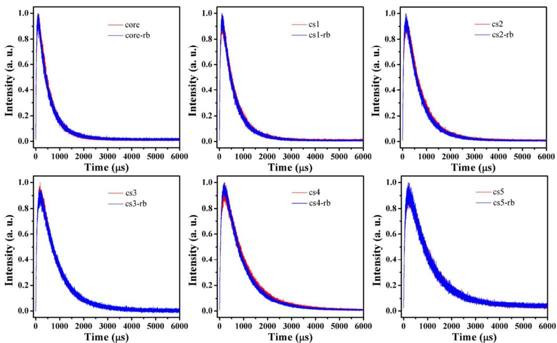
**Figure S2.** Temporal behavior of upconversion luminescence of UCNPs (red curves) and UCNPs-RB (blue curves) at 650 nm under 980 nm excitation.
