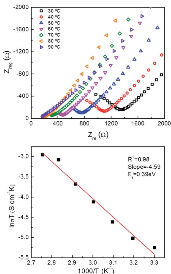
Fig. 4 Nyquist plots measured at 44% relative humidity and different temperatures (top) and the corresponding Arrhenius plot (bottom) for the NdMo-MOF activated at 80 °C.
