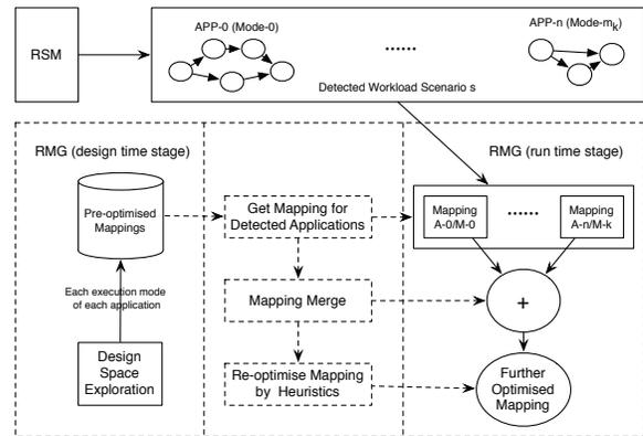
Figure 3: Mapping generation in the RMG component.
