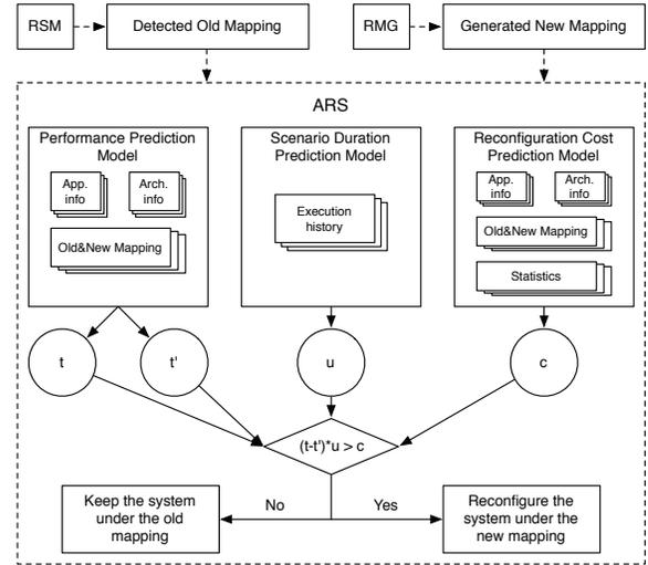
Figure 4: Overview of adaptive system reconfiguration in ARS
