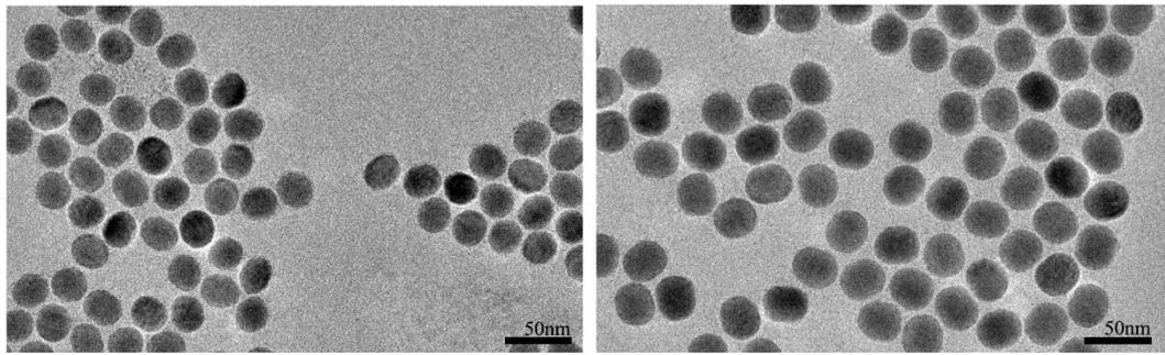
**Figure S1.** TEM images of core NaYF<sub>4</sub>: Yb, Er (left) and core-shell NaYF<sub>4</sub>: Yb, Er/NaYF<sub>4</sub>: Yb, Tm UCNPs (right).
