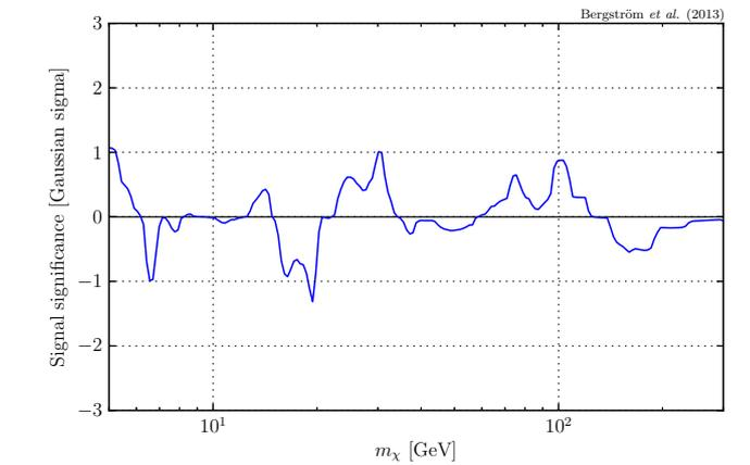
FIG. S3. Significance for a contribution from a  $e^+e^-$  DM signal to the AMS-02 positron fraction, for different DM energies, in units of Gaussian sigma. Negative values correspond to negative (but unphysical) signal normalizations.
