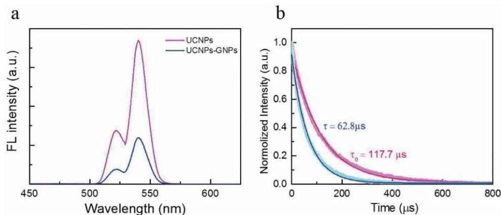
**Fig. S5.** (a) Upconversion fluorescence spectra of UCNPs (pink) and UCNPs-GNPs complex (blue) under 980 nm excitation; (b) the fluorescence decay curves of down-conversion emission monitored at 542 nm under 488 nm excitation and best-fitted curves for UCNPs (pink) and UCNPs-GNPs complex (blue)
