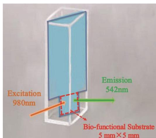
**Fig. S2.** The schematic diagram of the instrumental setup.
