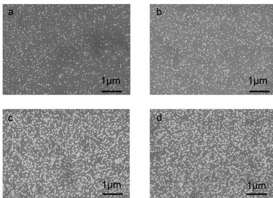
**Fig. S3.** SEM images of the silicon wafer substrates modified with UCNPs with different time, (a) 8 h, (b) 12 h, (c) 24 h and (d) 36 h.
