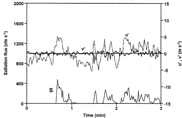
Figure 6. Saltation flux ( $S$ ) in relation to horizontal ( $u'$ ) and vertical ( $v'$ ) turbulent velocity fluctuations during the first 3 min of a storm event at ICRISAT Sahelian Centre on 25 June 1995
