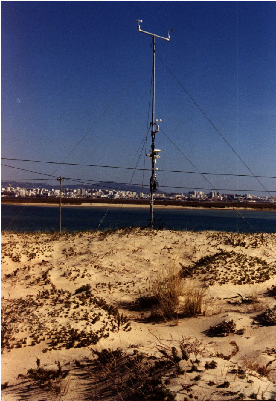
Figure 2. The dune crest with typical vegetation cover and mast with cupanemometers, wind vane and psychrometer.
