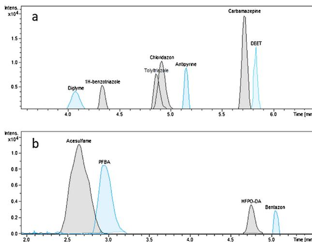
**Fig. 3.** Overlaid EICs of target analytes that could be quantified (grey) and those that were detected, albeit at concentrations below MQLs (blue) in non-spiked surface water samples analyzed in positive ESI mode (a) and negative ESI mode (b). (For interpretation of the references to colour in this figure legend, the reader is referred to the web version of this article).
