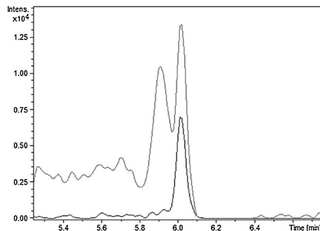
**Fig. 2.** EICs of ibuprofen (grey)  $m/z$  205.1234  $\pm$  0.002 and its bbCID MS/MS fragment  $m/z$  161.1330  $\pm$  0.005 (black) in a RBF sample spiked to 50 ng/L and extracted with SPE. The quasi-isobaric interference in the full-scan data can be seen at  $t_R$  5.9 min.
