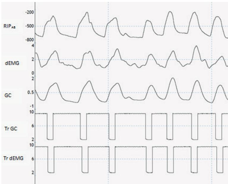
**Figure 1.** Example of a final recording file after triggering by the Infant Flow<sup>®</sup> SiPAP<sup>™</sup> system. RIP<sub>AB</sub>, respiratory inductance plethysmography abdominal belt; dEMG, transcutaneous electromyography of the diaphragm; GC, Graseby capsule; Tr GC, trigger of the Infant Flow<sup>®</sup> SiPAP<sup>™</sup> system based on the GC signal; Tr dEMG, trigger of the Infant Flow<sup>®</sup> SiPAP<sup>™</sup> system based on the dEMG signal.
