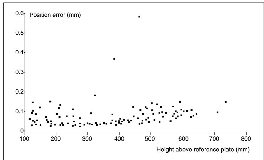
Figure 3. The Estimated rms Position Errors ( $\sigma_x^2 + \sigma_y^2 + \sigma_z^2$ ) for a Collection of 124 Images, as a Function of the z-height of the Camera. Notice that the Position Error Increases with the Height above the Reference Plate
