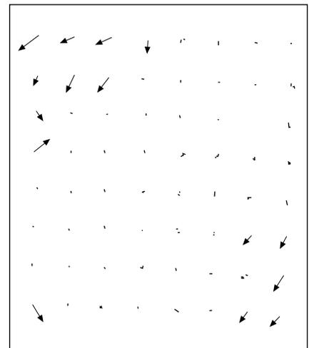
Figure 1. Residuals between Calculated and Measured Image Points, with a Six-parameter Camera Model (20x)
