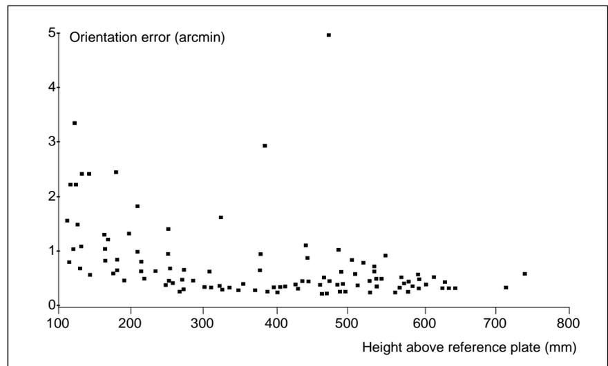
Figure 4. The Estimated rms Angle Errors ( $\sigma_\alpha^2 + \sigma_\beta^2 + \sigma_\gamma^2$ ) for a Series of 124 Images, as a Function of the z-height of the Camera. For the Range of z-heights Shown, the Orientation Error is Mostly Independent of z. It Tends to Increase for Small Values of z, as Fewer Reference Points Will be Visible
