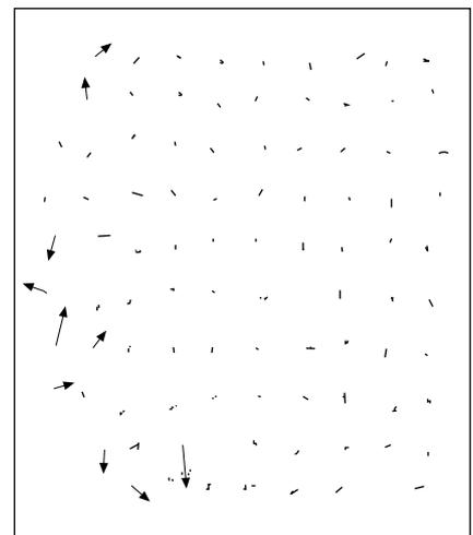
Figure 2. Residuals between Calculated and Measured Image Points, with a Nine-parameter Camera Model (200x)
