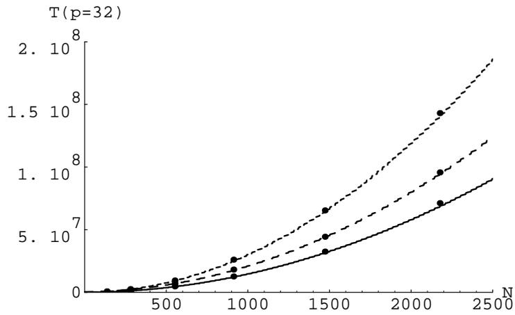
**Fig. 4.** The execution time (in  $\mu\text{s}$ ) on 32 processors, for one Conjugate Gradient iteration, as a function of the number of dipoles  $N$ ; the dots are the measurements, the lines are the theoretical predictions; solid line for Parix, short-dashed line for Iserver-Occam, and long-dashed line for Express.
