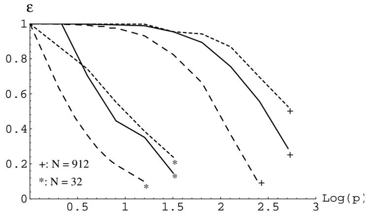
**Fig. 3.** The efficiency of a total Coupled Dipole simulation (including I/O), as a function of the number of processor, for  $N = 32$  and  $N = 912$ ; the solid line is for Parix, the short-dashed line for Iserver-Occam, and the long-dashed line for Express.
