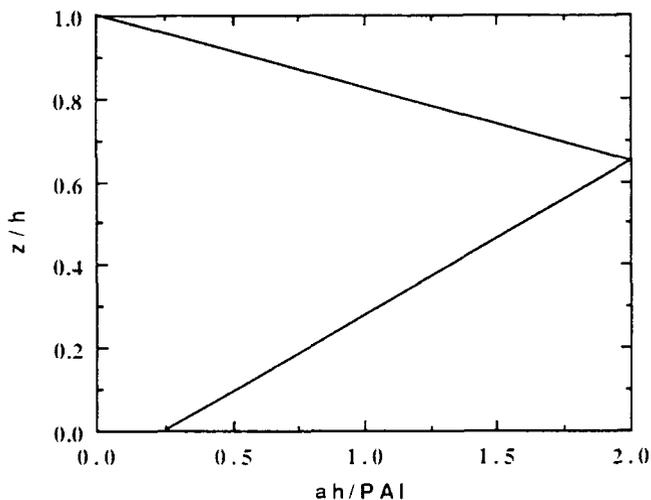
Fig. 1. The plant area distribution,  $a$ , i.e. one-sided plant area per volume air ( $\text{m}^2 \text{m}^{-3}$ ) nondimensionalized with the canopy height,  $h$ , and scaled with the plant area index PAI vs. the nondimensional height,  $z/h$ . The area under the curve is equal to unity with regard to the  $y$ -axis.
