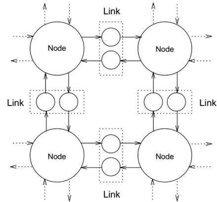
Figure 4: The base topology model for communication.
