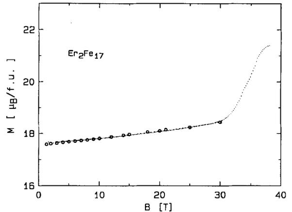
Fig. 5. Magnetization at 4.2 K of a spherical  $\text{Er}_2\text{Fe}_{17}$  single crystal free to rotate in the applied magnetic field [13]. The circles represent measurements in quasi-stationary fields and the dotted line corresponds to a measurement in a field increasing in an uncontrolled way and decreasing linearly with time at a rate of 50 T/s.
