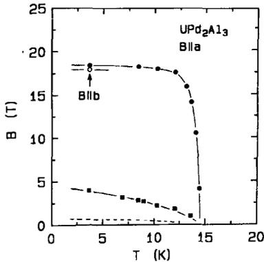
Fig. 10. Antiferromagnetic phase diagram of  $UPd_2Al_3$  for  $B||a$ . The dashed line is taken from Ref. [27]. The open circle denotes the antiferromagnetic phase boundary for  $B||b$ . The middle phase line (closed squares) is absent for  $B||b$ .
