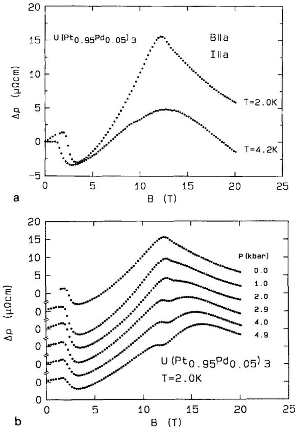
Fig. 8. (a) The magnetoresistance data for  $\text{U}(\text{Pt}_{0.95}\text{Pd}_{0.05})_3$  for  $B \parallel I \parallel a$  at 2.0 K (■) and 4.2 K (●). (b) Magnetoresistance data for  $\text{U}(\text{Pt}_{0.95}\text{Pd}_{0.05})_3$  for  $B \parallel I \parallel a$  at 2.0 K under hydrostatic pressures up to 4.9 kbar as indicated.
