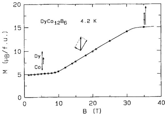
Fig. 4. Free-powder magnetization curve at 4.2 K of  $\text{DyCo}_{12}\text{B}_6$  [9]. The circles represent measurements in quasi-stationary fields and the full line corresponds to a measurement in a field decreasing linearly with time at a rate of 50 T/s. The moment configurations in the different field intervals are indicated.
