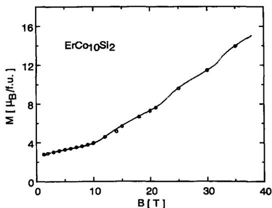
Fig. 6. Free-powder magnetization curve at 4.2 K of  $\text{ErCo}_{10}\text{Si}_2$  [14]. The circles represent measurements in quasi-stationary fields and the dotted line corresponds to a measurement in a field decreasing linearly with time at a rate of 50 T/s.
