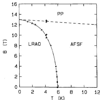
Fig. 7. The magnetic phase diagram of  $\text{U}(\text{Pt}_{0.95}\text{Pd}_{0.05})_3$  for  $B||a$ . Data are taken from specific heat ( $\square$ ), magnetization ( $\triangle$ ) and magnetoresistance ( $\circ$ ). LRAO denotes long-range antiferromagnetic order, AFSF denotes antiferromagnetic short-range correlations and PP denotes the polarised paramagnetic state.
