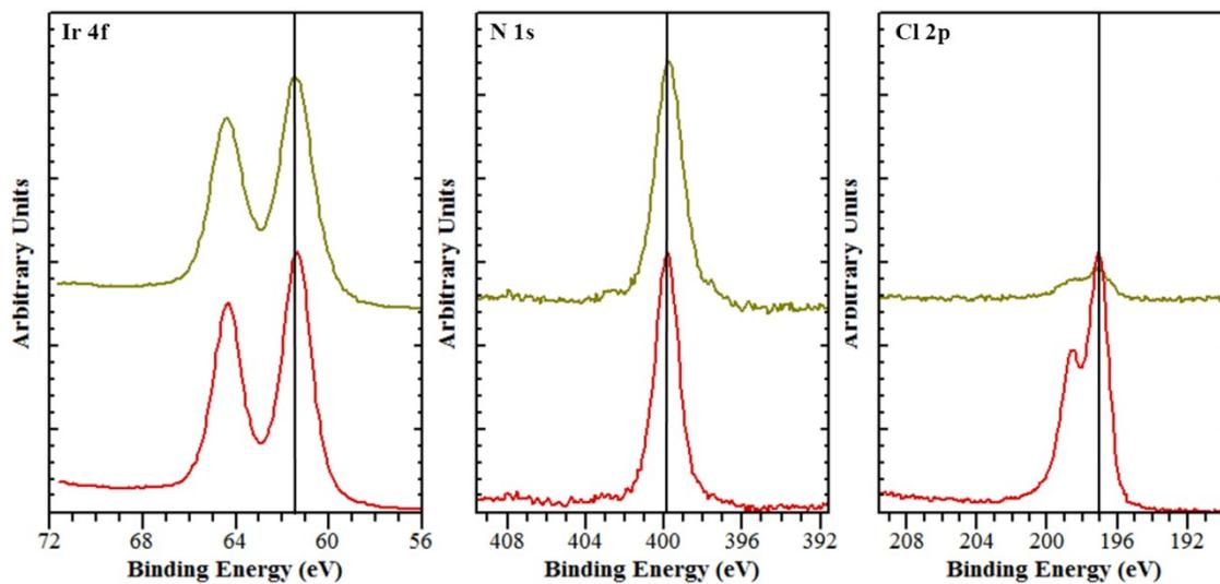
**Figure S4.** Iridium 4f, nitrogen 1s and chloride 2p XPS signals of **3** (red) and **1** (olive) powders. The lines indicate a binding energy of 61.4 eV for iridium, 399.8 for nitrogen and 197.1 for chloride. A trace of chloride was also observed in the sample of **1**, even though chloride analysis of the same batch by elemental analysis did not show any chloride content.
