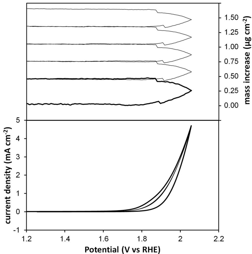
**Figure S3.** EQCM experiment wherein the mass balance (top) and current density (bottom) are simultaneously followed as a function of applied potential in case of a 1 mM solution of **1** in 100 mM  $\text{Na}_2\text{HPO}_4$  on a gold electrode. The first scan is depicted in bold. Phosphate is an inhibitor of catalytic activity mediated by **1**.
