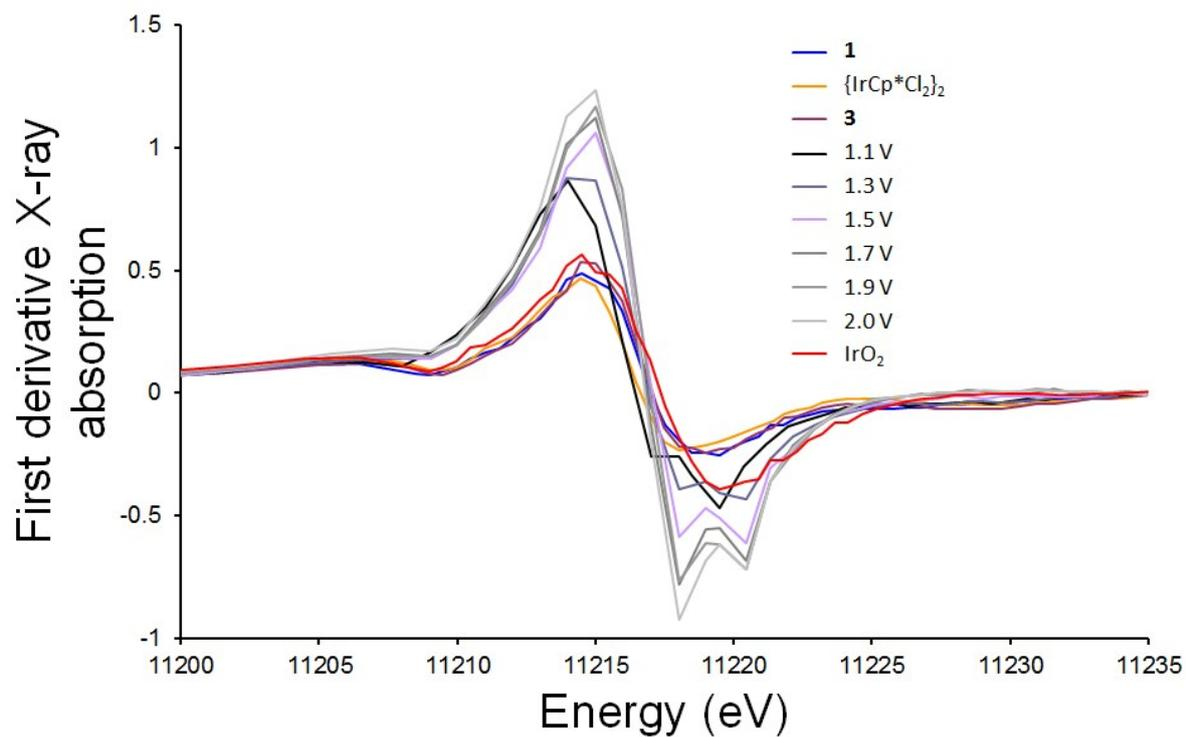
**Figure S7.** First derivative of the X-ray absorption at the iridium L<sub>3</sub> edge for selected reference complexes **1**, **3**, (IrCp\*Cl<sub>2</sub>)<sub>2</sub> and IrO<sub>2</sub> as well as **DM**|GC prepared at 1.1 V, 1.3 V, 1.5 V, 1.7 V, 1.9 V and 2.0 V versus RHE.
