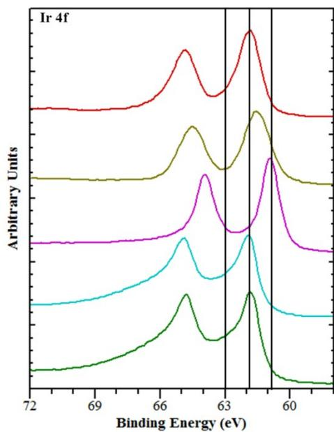
**Figure S6.** Iridium 4f XPS signals of IrCl<sub>4</sub> • x H<sub>2</sub>O (red), Iridium(III) 2,4-Pentadionate (olive), iridium foil sputtered (purple), iridium foil calcined (blue) and calcined IrCl<sub>3</sub> • x H<sub>2</sub>O (green) yielding binding energies of 60.7 eV for metallic iridium and 61.8 eV for Ir<sub>2</sub>O<sub>3</sub>. IrO<sub>2</sub> has a binding energy of 63.0 eV.
