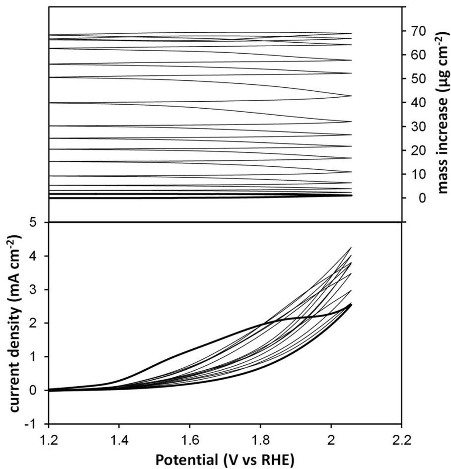
**Figure S2.** EQCM experiment wherein the mass balance (top) and current density (bottom) are simultaneously followed as a function of applied potential in case of a 1 mM solution of **1** in 100 mM  $\text{Na}_2\text{SO}_4$  (non-buffered) on a relatively rough gold EQCM electrode. The first scan is depicted in bold.
