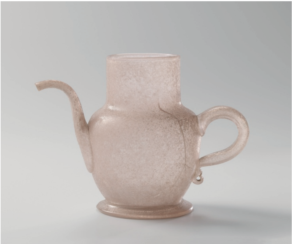
Figure 1.2. Fully crizzled and discoloured flagon with spout and ovoid body, height 13.9 cm, ca. 1700. Rijksmuseum, Reg. No. BK-NM-804. Photo: © Rijksmuseum.
