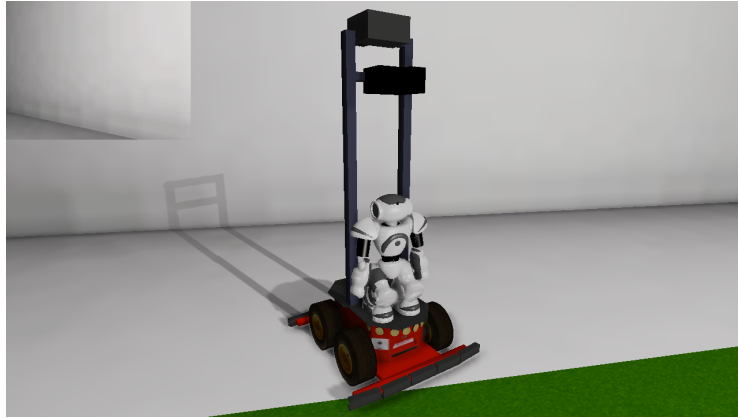
Fig. 1: Configuration of a humanoid robot on a wheeled platform in USARSim, as used in the RoboCup @Home [2].
