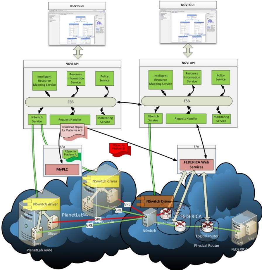
Fig. 1. NOVI Federated Data, Control & Management Architecture
