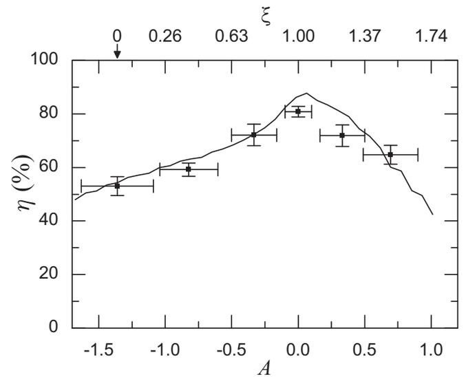
FIG. 6. Maximum single-path STIRAP efficiency as a function of the parameter  $A = \delta_m/\tilde{\gamma}$ , varied by changing the intensity  $I_{\text{COMP}}$  of the compensation beam. Values of the compensation level  $\xi$  are given on the top axis for reference. Theoretical values (line) are obtained by simulating the STIRAP process with Eq. (1), using independently determined parameters and not performing any fit. The error bars represent one standard deviation.
