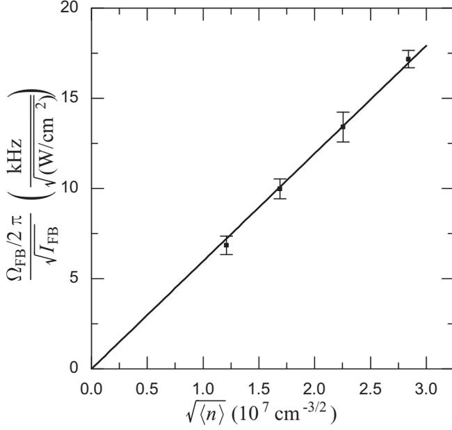
FIG. 3. Free-bound Rabi frequency  $\Omega_{\text{FB}}$  as a function of  $\sqrt{\langle n \rangle}$ , where  $\langle n \rangle$  is the average on-site density of a single atom. The line is a linear fit to the data, justified in the text.
