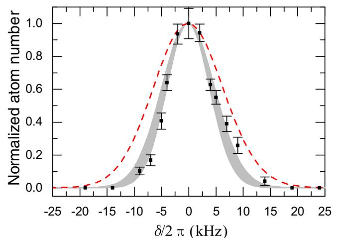
FIG. 11. Dependence of STIRAP efficiency on the two-color detuning  $\delta$ . The data points show the normalized number of atoms retrieved after two STIRAP cycles. The red dashed line is the shape determined by our model for  $\gamma_e = \Gamma_e = 2\pi \times 17.0(1.5)$  kHz, while the gray area spans the widths between  $2\pi \times 30$  kHz and  $2\pi \times 57$  kHz, which are the fitted values for the positive-detuning and the negative-detuning side, respectively.
