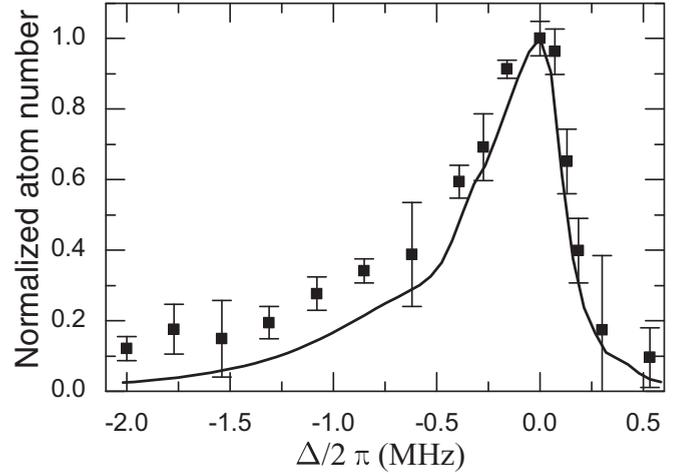
FIG. 10. STIRAP efficiency in dependence of the one-color detuning  $\Delta$ . The data points show the normalized number of atoms retrieved after two STIRAP cycles, depending on the value  $\Delta$  used for the second STIRAP. The solid line is derived from Eq. (1) using no fit parameters.
