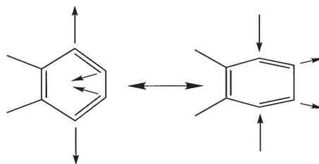
**Fig. 6.** The in-plane C–C–C bending of the pendant ring that characterizes vibrational modes near 16  $\mu\text{m}$ . The intensity at this position involves an in-phase, planar vibration of the two opposite carbons of the pendant ring (i.e. at the para positions) along the line which is parallel and adjacent to the fused bond with the rest of the molecule's carbon network.
