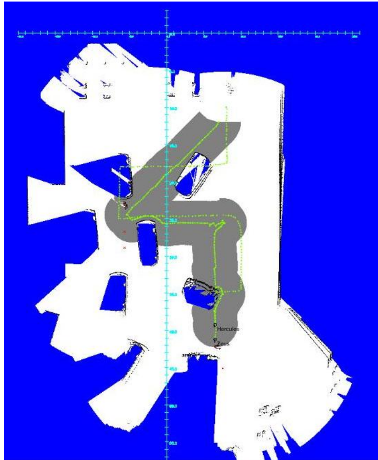
Fig. 3. Map generated by the ground robot in the outdoor area of CompWorldDay1
