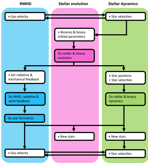
Figure 1. Flowchart showing the order of operations and information passed between the codes handling RMHD (left, FLASH), stellar and binary evolution (center, SEBA), and stellar dynamics (right, PETAR), for one TORCH time step. The boxes with a white background denote updates from one code to another, while the boxes with a darker background correspond to operations done within one code.
