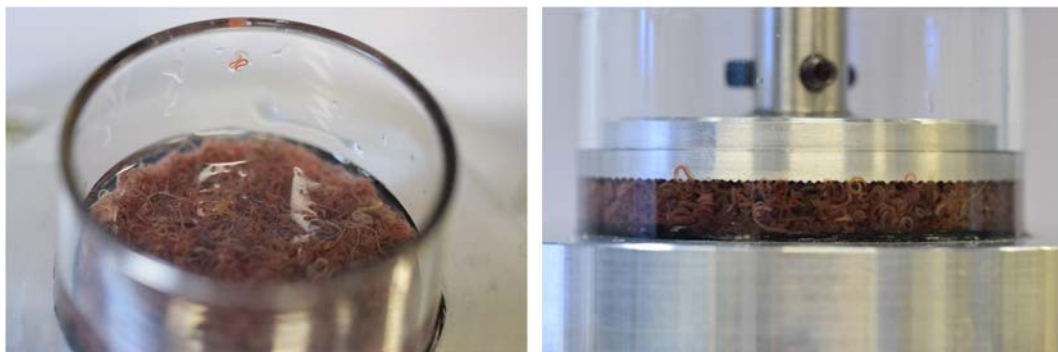
Fig. 3. (Left) A known mass of worms is mixed with water and placed in a custom designed rheology cell. (Right) The rough plate-plate rheology cell allows us to perform rheology measurement on the living worm suspension.
