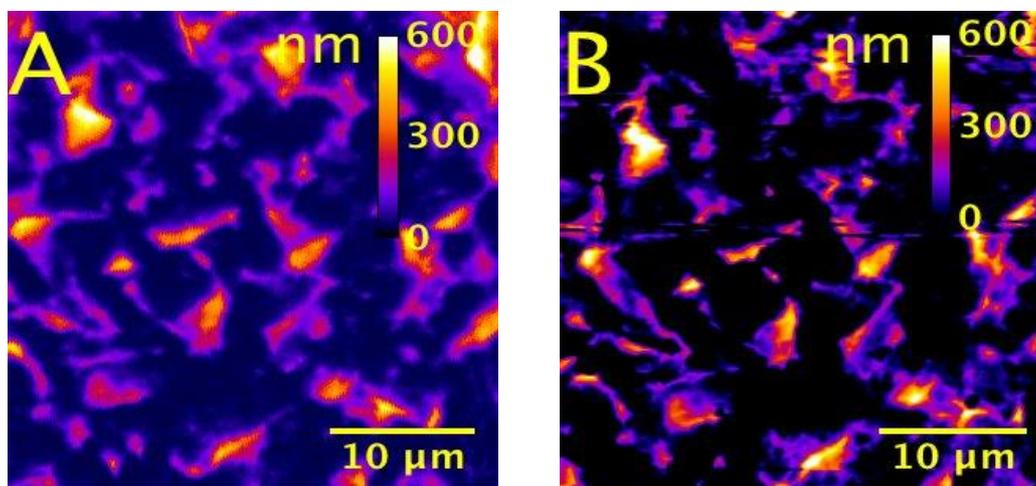
Figure S4. Rough PS sphere on smooth glass coverslip interface. For ease of visual comparison, zoomed areas of the overall surface are shown. A) Image obtained by the fluorescent liquid method. B) AFM image of the same PS bead. The height values in A) do not go down to zero because a thin boundary layer of the fluorescent liquid separates the two surfaces.
