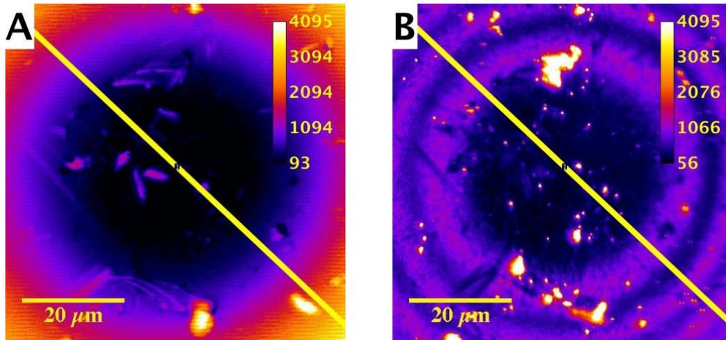
Figure S2. Contact area between the glass bead and a glass coverslip imaged with fluorescent liquid method. The cross-section for calibration of the scaling factor is indicated in each of the images. a) Fluorescence intensity image. b) Reflection of the laser light forming an interference pattern of Newton rings.
