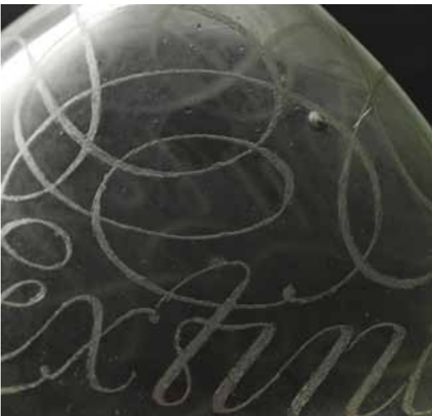
Fig. 2. (top) Dutch engraved glass flask, height 17.6 cm, ca. 1675–1692 (Rijksmuseum Amsterdam, Reg. No. BK-NM-754). (bottom) Detail showing surface deterioration, assigned to category D (Photo: © Rijksmuseum).
