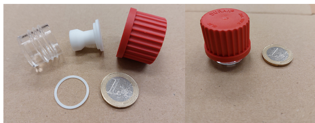
Figure 2. Photos of its individual parts and a fully assembled liquid cell. A euro coin is added as a scale reference. The glass vial, PTFE insert, PTFE spacer, and PBT with glass fiber cap are visible on the left. After liquid is added to the glass container, the insert and spacer are positioned, after which the cap is used to close the cell as depicted on the right.
