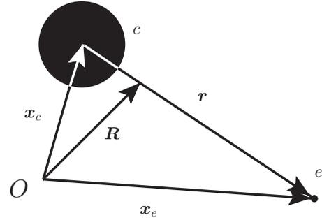
FIG. 1. Schematic of the coordinates used in this paper.  $O$  denotes the origin.  $\mathbf{x}_e$  and  $\mathbf{x}_c$  are the position vectors of the electron and core, respectively, in the Ioffe-Pritchard frame.  $\mathbf{r}$  and  $\mathbf{R}$  denote the relative and center-of-mass coordinates, respectively. Since the mass is almost entirely contained in the core we approximate  $\mathbf{R}$  with  $\mathbf{x}_c$ .
