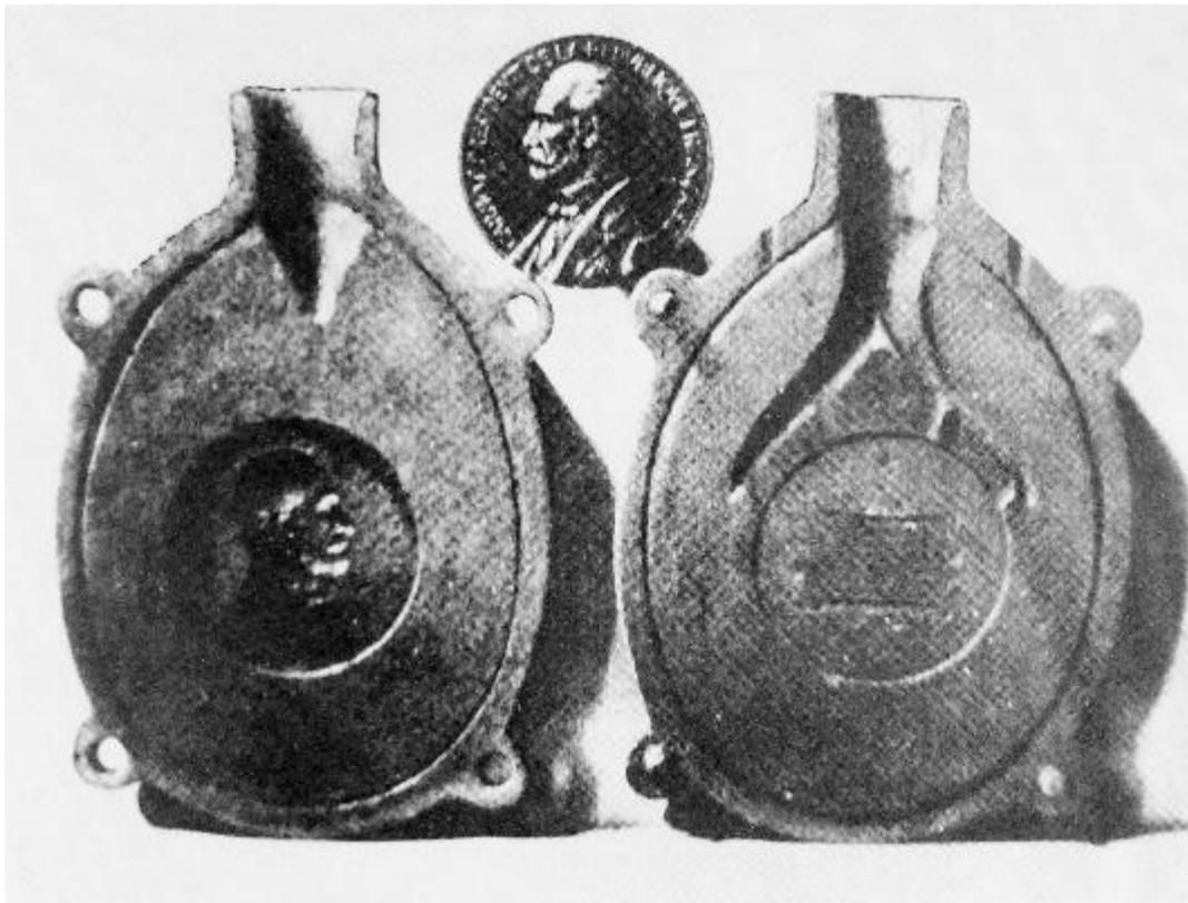
Fig. 1.9. A finished sand mould inside a flask ready for casting. The medal used as pattern has been removed and the gating system has been carved in the surface of the sand. (from Richter, Ernst-Ludwig. *Altes Silber*, Keyser, 1983, fig. 201)
