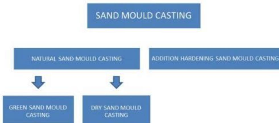
Fig. 1.2. Diagram illustrating the various sand mould casting methods.
