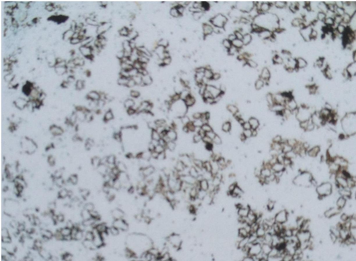
Fig. 1.3. Petrographic sample illustrating core material with loose sand grains of roughly equal size, each outlined by a thin layer of dark clay. The clay shows up as a dark line around each individual sand grain. Core sample from *Hercules, Nessus, and Deianeira* (Rijksmuseum Amsterdam, inv.no. BK-1957-2), cast attributed to Crozatier, design after Adriaen de Vries, sand mould casting, probably Paris c.1845-1850. ( from Bassett and Schmidtling II 2012, 38)
