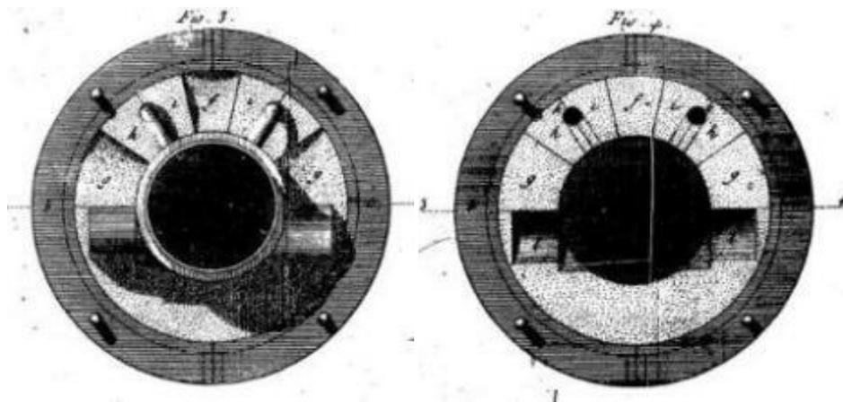
Fig. 1.23. Detail from plate XIII *Moulage en Sable* from Monge's treatise on gun founding, illustrating a cross section of cannon mould showing the use of piece-moulding with false cores. This enabled the moulding of the handles and trunnions of the cannon using sand moulds: Monge 1793-94.
