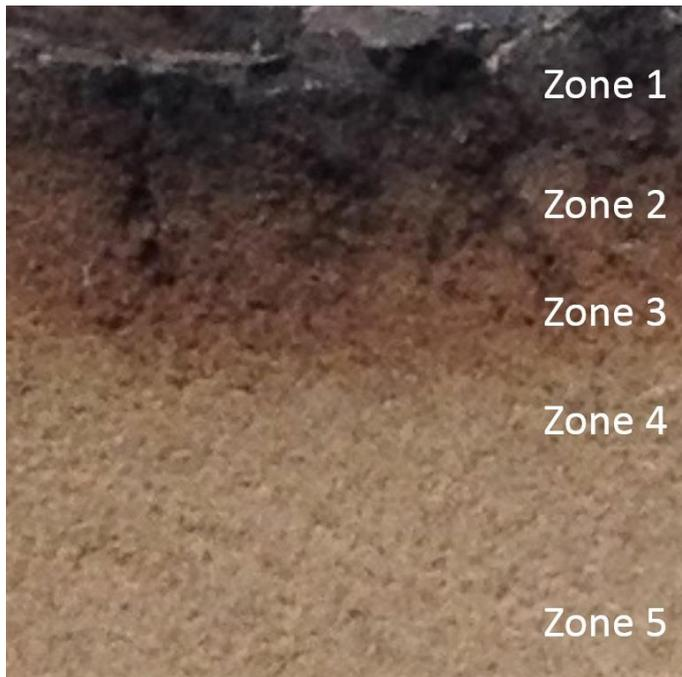
Fig. 1.6. Close up of the cross section of the heat affected mould surface with the five zones indicated.
