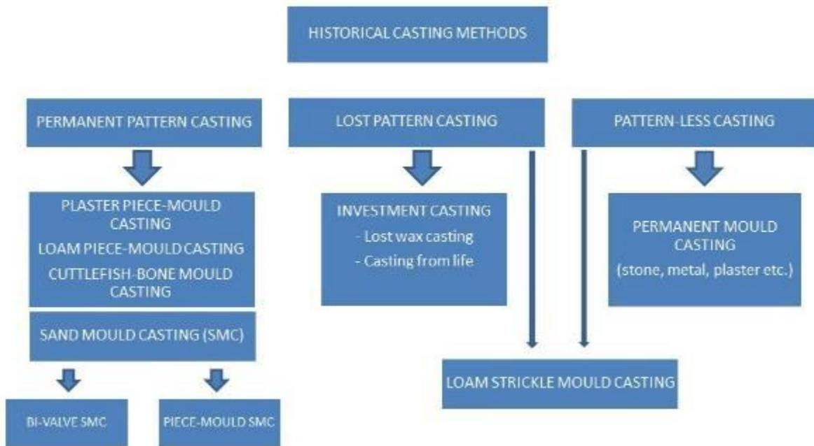
Fig. 1.1. Historical casting ‘family tree’, arranging the main casting methods in use before 1900.
