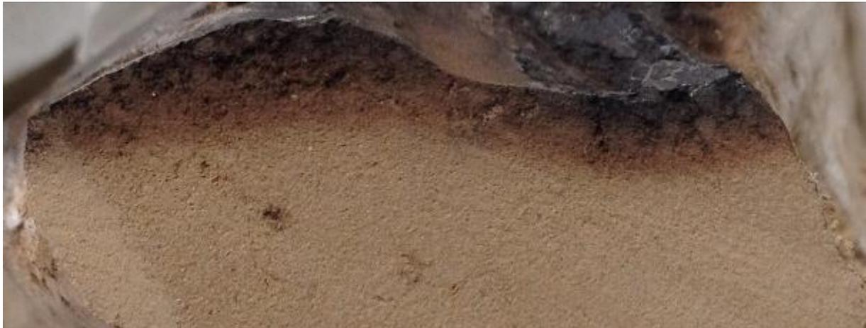
Fig. 1.5. Cross section of a reproduction outer mould section of Brussels earth, showing the visible effect of the heat of the molten metal.
