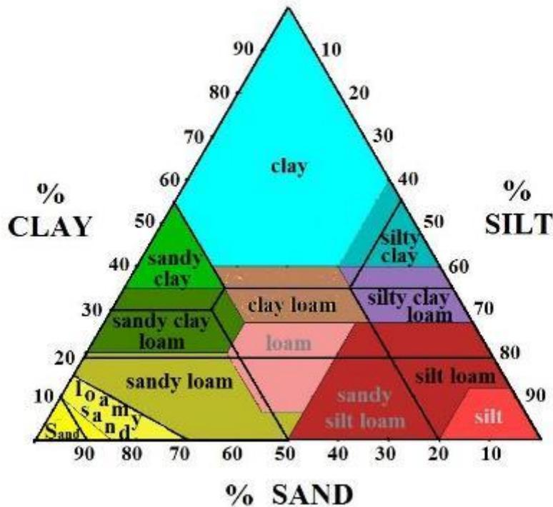
Fig.1.4: Soil textural triangle showing both the USDA and the UK-ADAS soil classes. (image Wiki commons)
