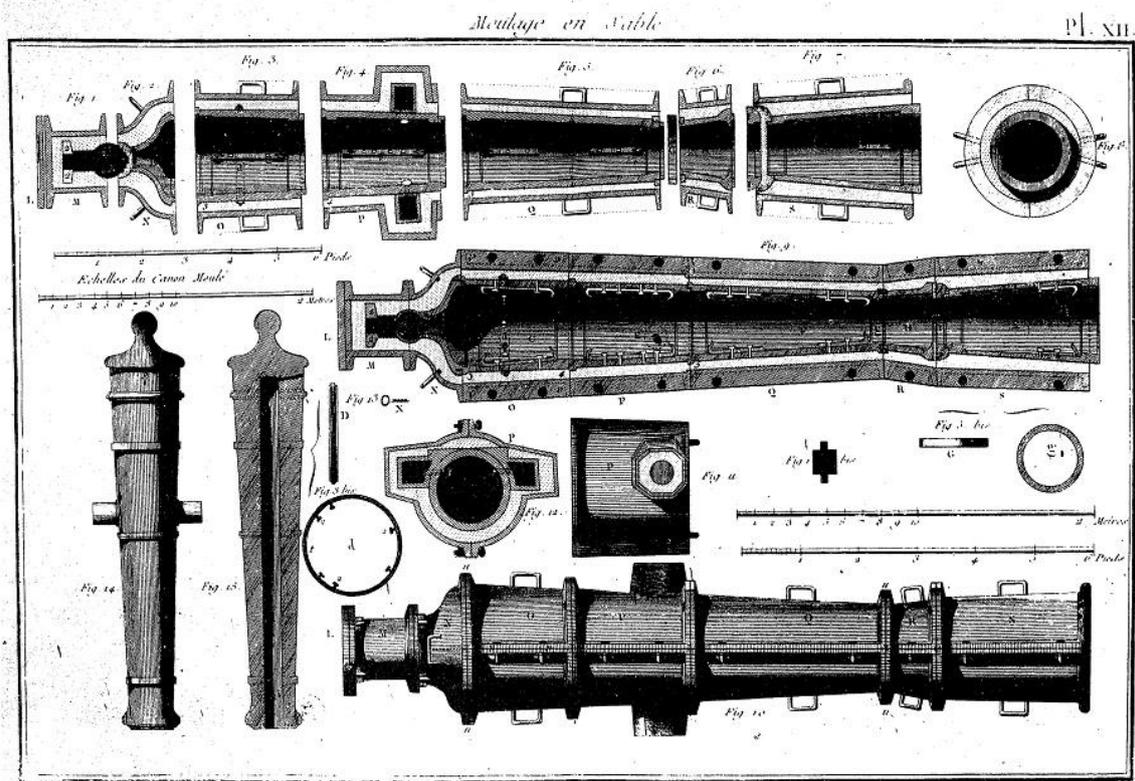
Fig. 1.22. Engraved plate XIII from Monge's treatise on gun founding. Illustrating the assembly of flasks to form the complete cannon mould from Gaspar Monge; *Description de l'art de fabriquer les canons*. Paris: L'Imprimerie du Comité de Salut Public, 1793-94
