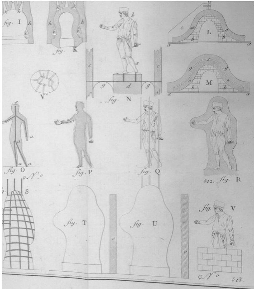
Fig. 2.17. Engraving illustrating various stages in the lost wax moulding and casting of a statue, plate 35 from Hassenfratz, *Siderotechnie*, 1812, Vol 2.
