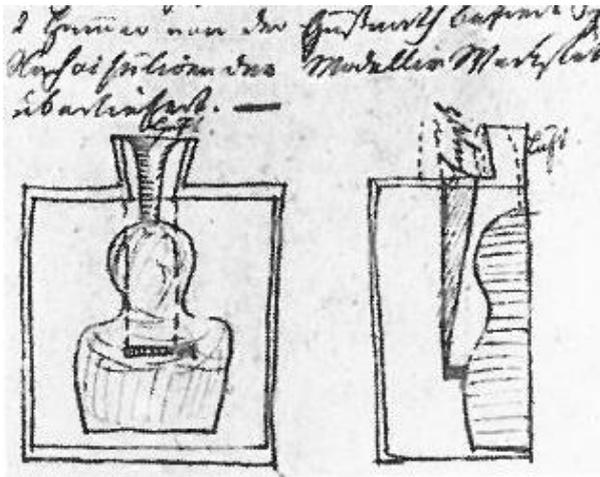
Fig. 2.10. Unknown artist, drawing c.1820, illustrating the pattern for the *bust of Werner* on the moulding board with the false core indicated with the dotted line. Also visible is the wedge shaped wooden pattern for the main sprue (from Vorsteher, 1982, 266).
