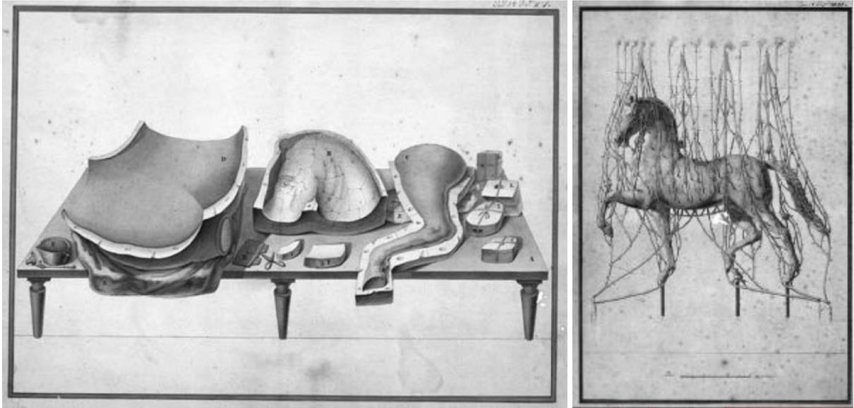
Figs. 2.23 & 2.24. Foundry S. Giorgio a Cremano (Righetti foundry Naples), left figure; preparation of wax model in plaster piece-moulds, note the scissors for cutting the wax plates. pl. n. 12, fig. XV. Right figure; the gating system attached to the wax model of the horse, pl. n. 18, fig. XXII. Both illustrations are pen drawing and watercolor, ASV, Instrumenta Miscellanea. (from Teolata, 2013)
