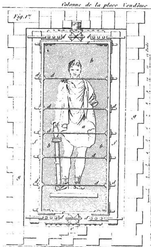
Fig. 2.3. Detail from plate IV from Launay foundry manual, depicting the statue of Napoleon by Chaudet, for the column at the Place Vendôme in Paris during moulding. Jean-Baptiste Launay, *Manuel du Fondeur*, Paris, 1827, volume I.
