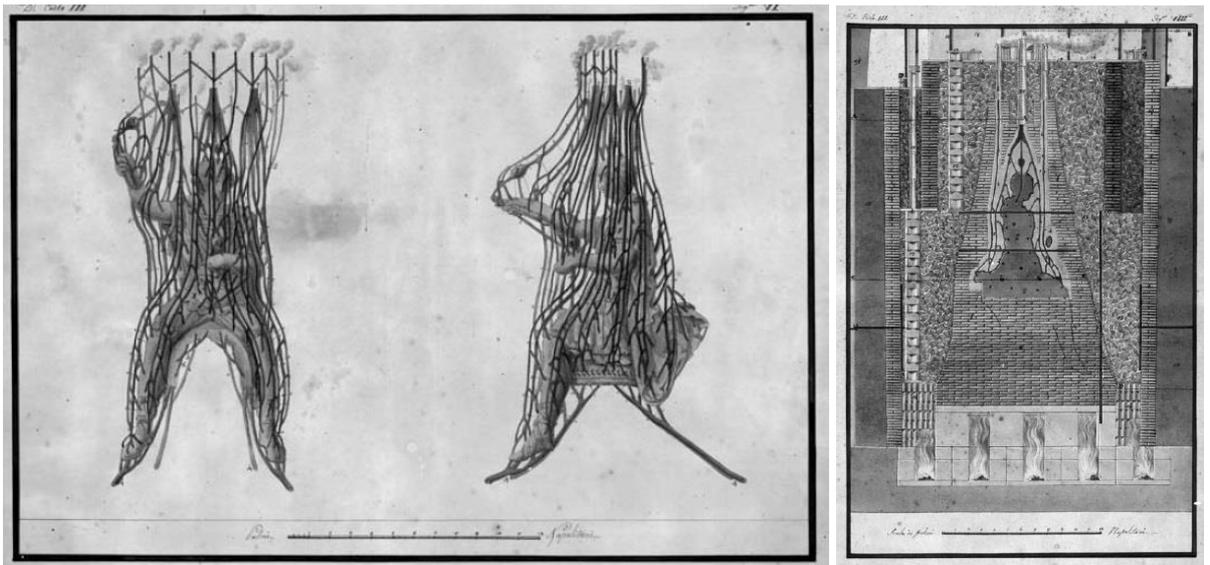
Figs. 2.25 & 2.26. Foundry S. Giorgio a Cremano (Righetti foundry Naples), left figure; Illustration of the gating system for the horseman indicating the system of runners and risers. Pl. n. 1, fig. VI. Right figure; cross section illustrating the set up for wax burn-out. Pl. n. 1, fig. VIII Both illustrations are pen drawing and watercolor, ASV, Instrumenta Miscellanea. ( from Teolata, 2013)
