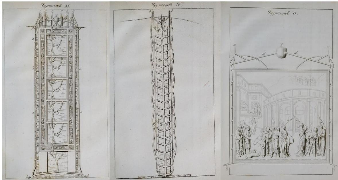
Fig. 2.18. Three plates (p.61, p.63, p.65 from Chekalevsky (1810) illustrating the gating system for the doors and one of its plaquettes for the cathedral of our lady of Casan in St. Petersburg.
