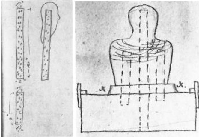
Fig. 2.11. Unknown artist, drawing c.1820, illustrating the lanterns(left) and their position within the core during the moulding of the *bust of Werner*. (from Vorsteher, 1982, 269).
