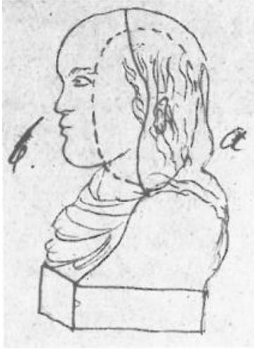
Fig. 2.9. Unknown artist, drawing c.1820, illustrating the pattern for the *bust of Werner* with the position of the false cores indicated with the dotted line (from Vorsteher, 1982, 267).
