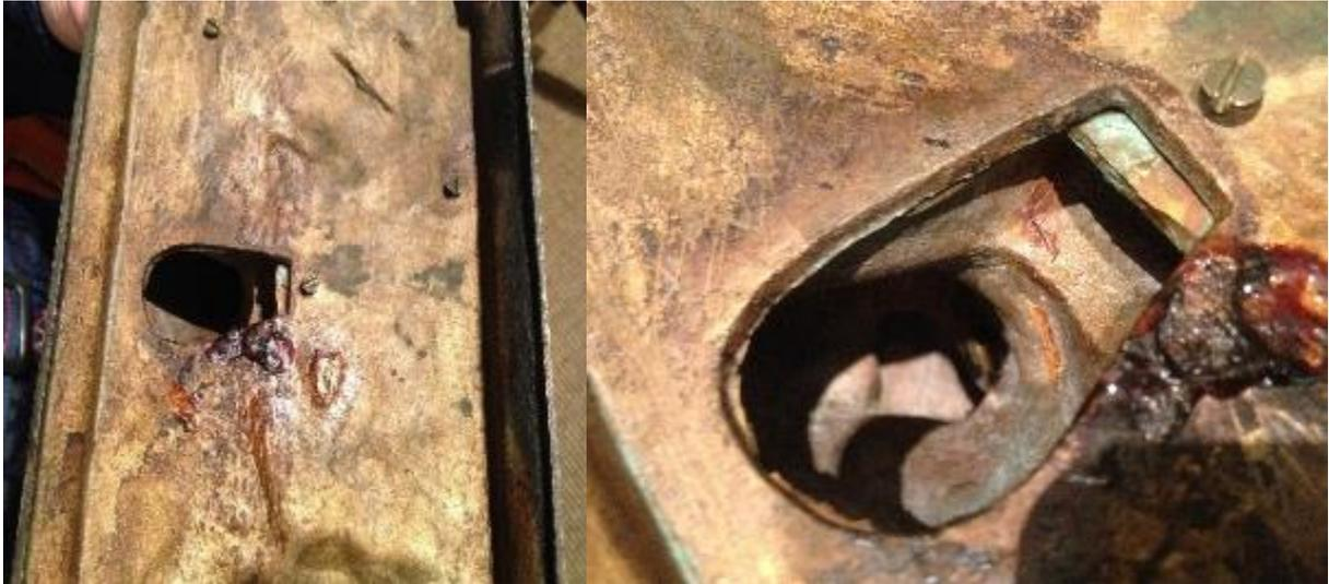
Fig. 2.13. Underside of the base of *Telephos*, illustrating the smooth sand mould cast surface with a wall thickness between 2-3 mm.
