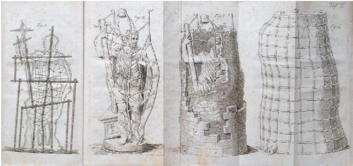
Fig. 2.19. Plate II from Wuttig illustrating various stages in the lost wax casting process. The four figures on this plate are exact copies of plates H, I, K, and L. from Chekalevsky treatise from 1810: Wuttig, *Die Kunst aus Bronze Kolossale Statuen zu Giessen*, Berlin.(1814)
