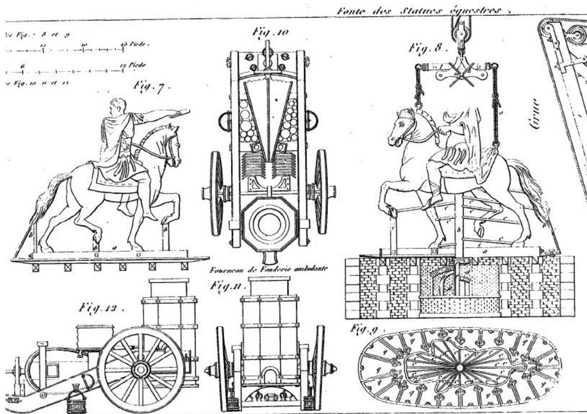
Fig. 2.7. *Fonte des Statues équestres*, illustrating the model and mould of an equestrian statue. Detail of plate 7 from Launay, *Manuel du Fondeur*, Paris, 1827, volume II
